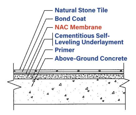
All NAC sheet membranes (ECB®, ECB® 75, Strataflex®, SAM® 3 and Super SAM® 125) may be used in this type of application for above-ground concrete substrates with a cementitious self-leveling underlayment.
