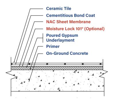
All NAC sheet membranes (ECB<sup>®</sup>, ECB<sup>®</sup> 75, Strataflex<sup>®</sup>, SAM<sup>®</sup> 3 and Super SAM<sup>®</sup> 125) may be use in this type of application with a poured gypsum underlayment.
