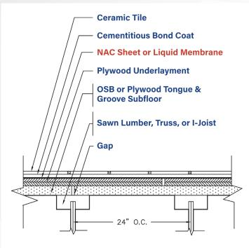
All NAC sheet membranes (ECB<sup>®</sup>, ECB<sup>®</sup> 75, Strataflex<sup>®</sup>, SAM<sup>®</sup> 3 and Super SAM<sup>®</sup> 125) may be used in this type of application for wood substrates in dry areas where the joist spacing is 24" on center or less.
