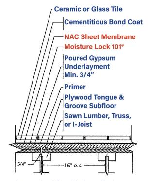
Use of a membrane is required for this installation.
