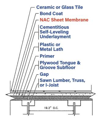
All NAC sheet membranes (ECB®, ECB® 75, Strataflex®, SAM® 3 and Super SAM® 125) may be used in this type of application for wood substrates with a cementitious self-leveling underlayment where the joist spacing is 19.2" on center.
