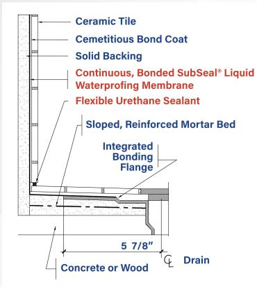
Shower receptors, curbs, seats, etc., must be properly waterproofed and installed to avoid water damage to adjacent building materials.
