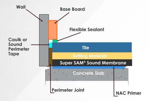
Perimeter joints are required at the edge of the floor area being treated and at any penetration of the floor inside of the perimeter, including where the base board meets the finished floor.
